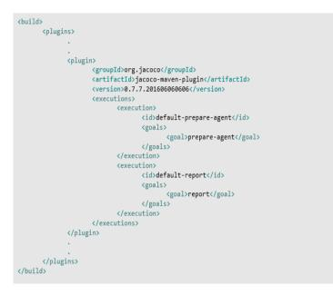
Fig 3: Adding Maven pom.xml dependency
